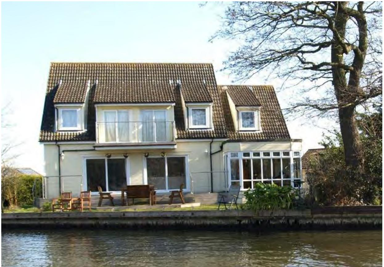
Above: A late 20<sup>th</sup> century chalet building of 1.5 storeys, with a steeply pitched roof containing accommodation, lit by dormers. The roof has concrete pantiles and the walls have a light-coloured render.
