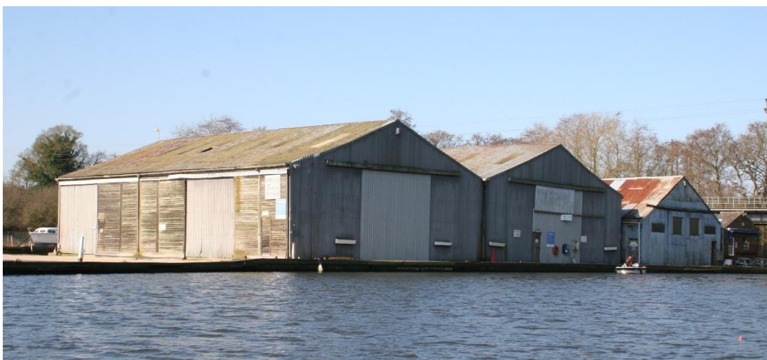
Above: typical boatyards in Barton Turf, Thorpe St Andrew and Wroxham (top to bottom), with large boatsheds of varying heights but similar forms with a prominent gable fronting the water's edge and the use of metal and timber cladding.
